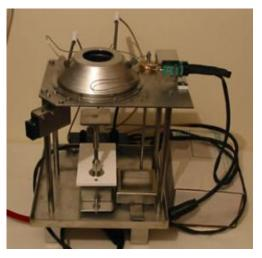
stability. The operator could have extra time to detect before the test start. If there is no opening closing mechanism, the flammable samples are easy to burn too early. So this extra time is very important for the operator.
