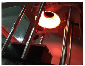
6.2, The burner correction system use purity of 99.5% methane to calibrate the instrument heat release rate; methane mass flow meter precise control of the flow of methane.
